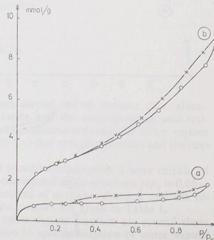
Fig. 4. Isotherms obtained for argon adsorption and desorption on zinc montmorillonite at 77.2 K
