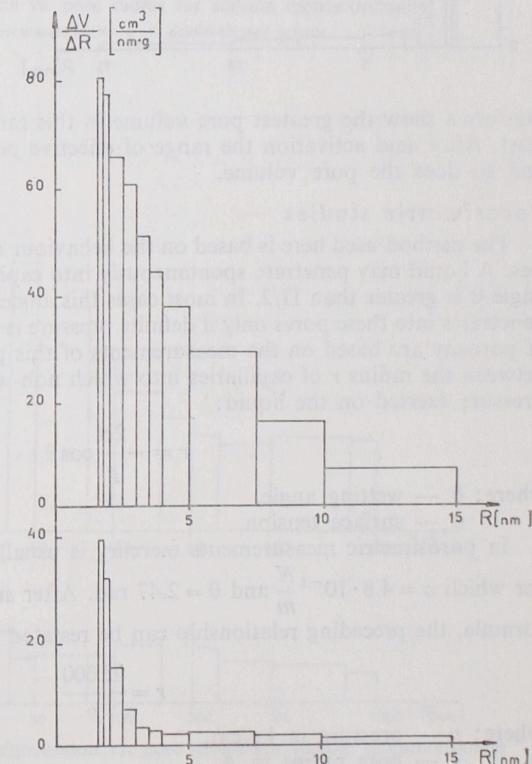
Fig. 6. Pore volume distribution vs. effective radius for sodium montmorillonite
