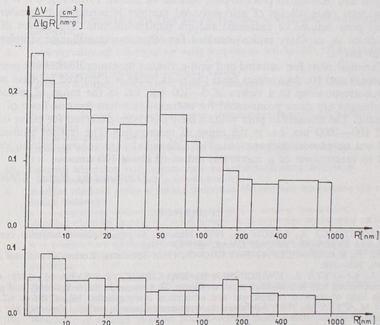
Fig. 9. Differential pore volume distribution vs. pore radius for sodium montmorillonite
