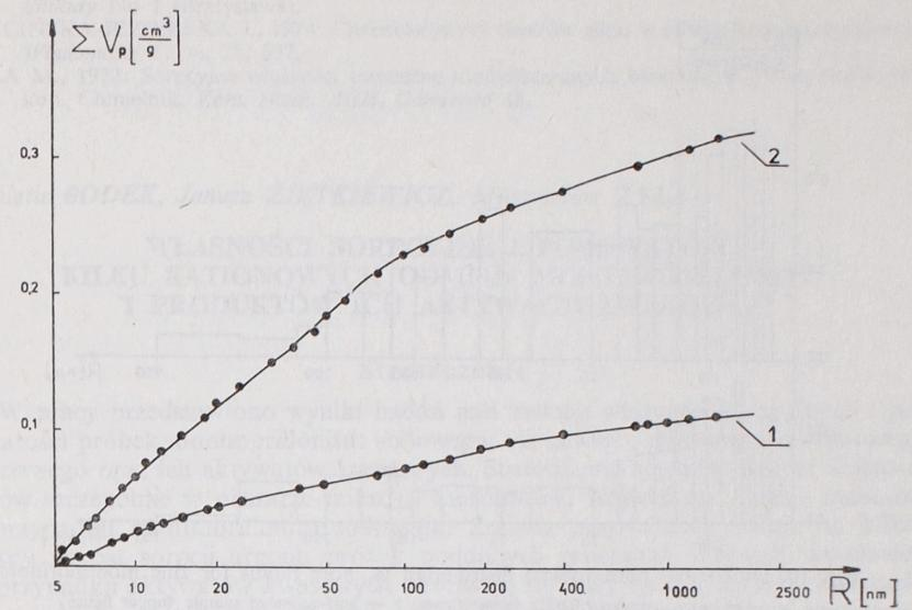
Fig. 8. Total pore volume vs. pore radius for sodium montmorillonite
