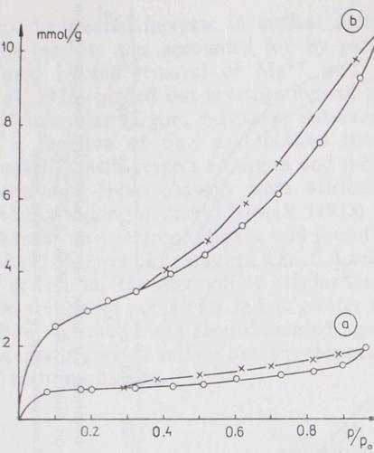
Fig. 3. Isotherms obtained for argon adsorption and desorption on sodium montmorillonite at 77.2 K
