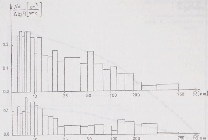
Fig. 10. Differential pore volume distribution vs. pore radius for zinc montmorillonite
