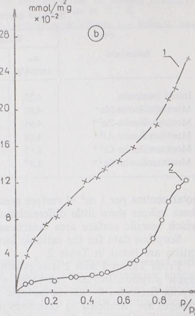
Fig. 5b. Absolute isotherms for water determined on zinc montmorillonite
