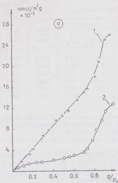
Fig. 5a. Absolute isotherms for water determined on sodium montmorillonite
