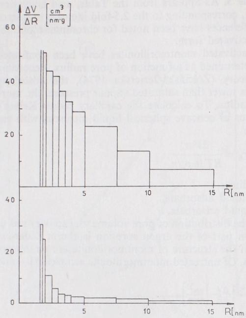
Fig. 7. Pore volume distribution vs. effective radius for zinc montmorillonite
